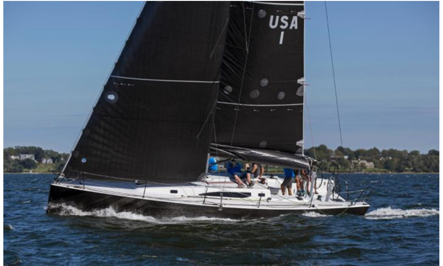
Non-Overlapping Jibs (Make sure that they all have the appropriate battens and are in the sail before the race if they are horizontal)
