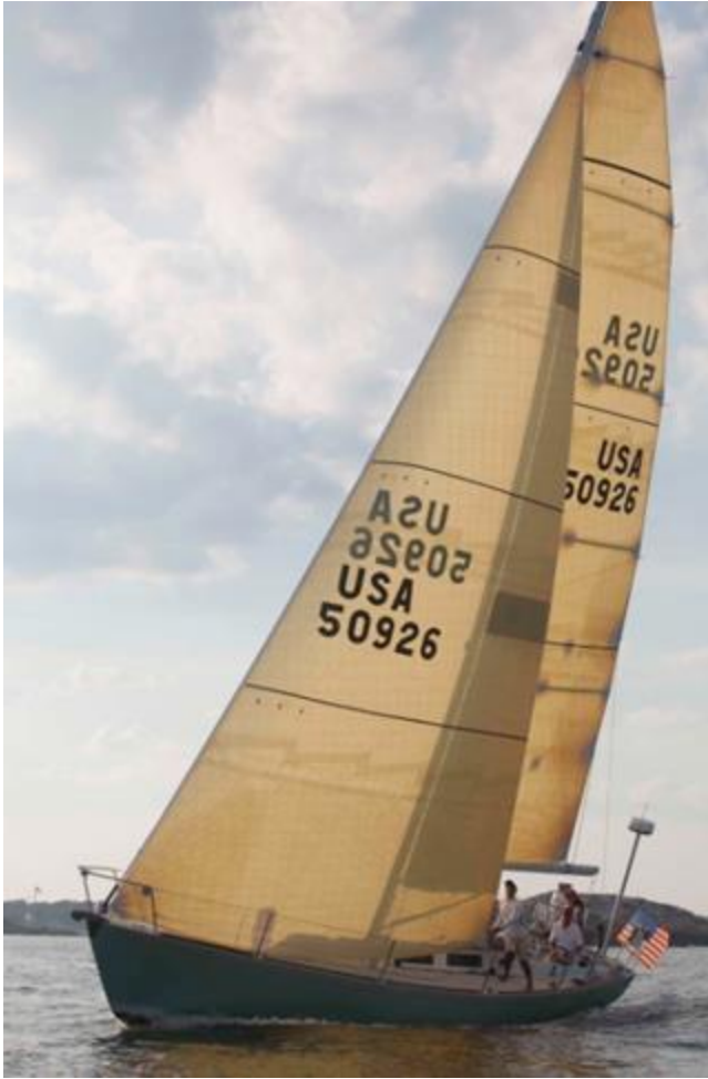
Overlapping Genoas (Tend to have more surface damage from tacking and hitting the rig)
